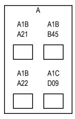
The above telecommunications outlet indicates that there are 3 cables coming from the A1B location, and 1 cable coming from A1C. The colour of the jack will indicate whether it is a data or other connection as per the jack colour coding requirements listed in **4.7.2.1 Colour Code Guidelines**. All of the telecommunications outlets must also be labelled with their position in the
