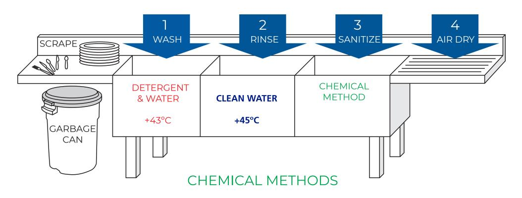
CHLORINE SOLUTION = 100 ppm Submerge for at least 10 seconds
